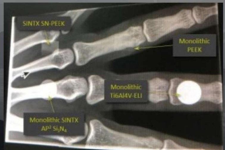
X-ray radiograph showing various biomaterials beneath a human hand as a demonstration of radiotranslucency (adapted from Pezzotti et al. 3 )
