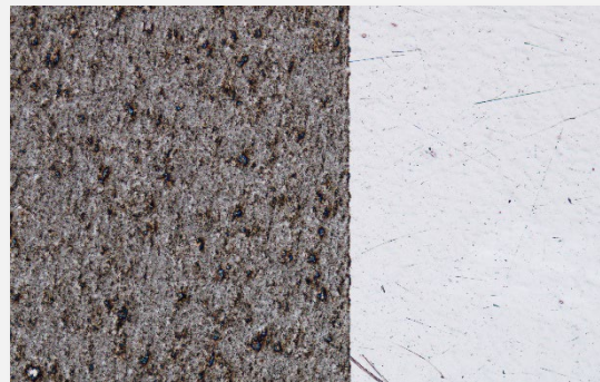
LEFT: Titanium surface laser clad with silicon nitride.
